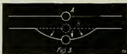
A, The Field About a Stationary, Electric Charge; B, The Way a Field Resists Motion, Or Its Inertia.
